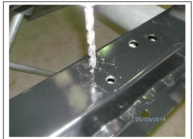
Figure 2: Enlarge two holes in rear of bumper support to 10mm.
