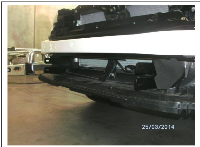
Figure 5: Mounts fitted to vehicle.
